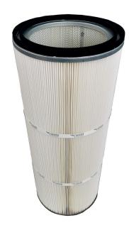
Camfil filter cartridge for the Quantum Series is manufactured using Dura-Pleat DPT spun bonded polyester media with PTFE membrane coating. It is integral to the Quantum Series units handling of thermal cutting processes from laser and plasma for superior filtration efficiency.
